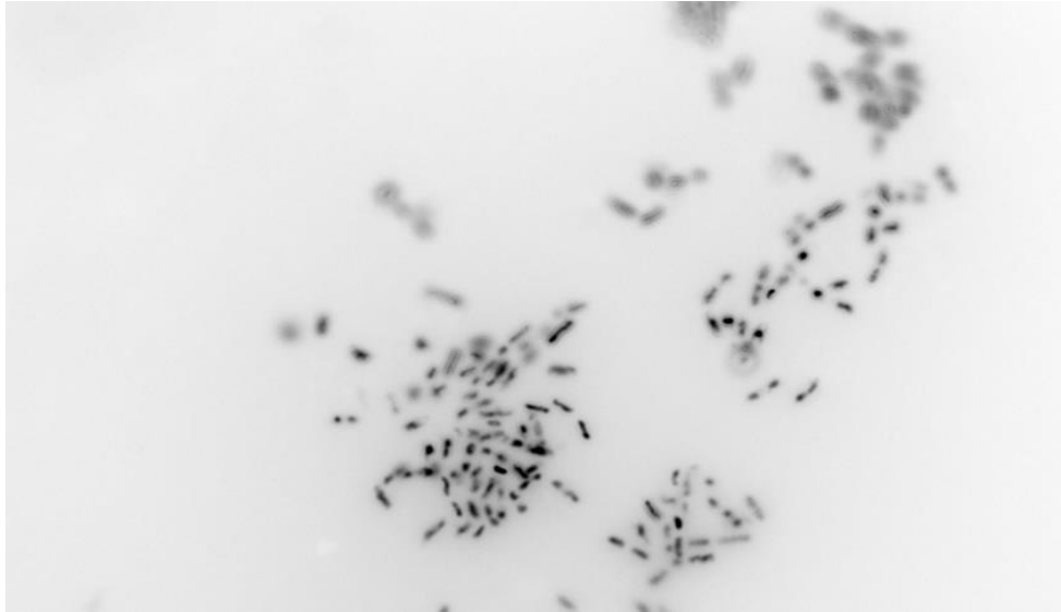
Images of extracted bacterial cells from non-spiked FEBEX clay sample B-C-60-18 after hydration
