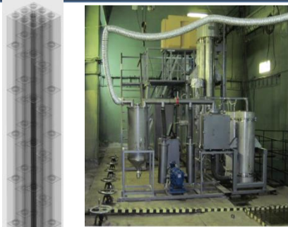
Pilot facilities for testing technology of i-graphite treatment
