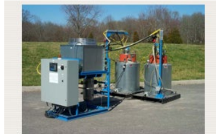
Unit for drying solids (IX resins, sludges, concentrates)
