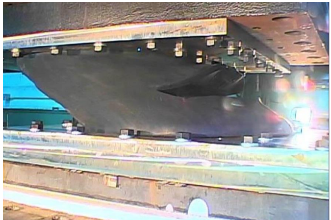
FIG. 6. Three-directional dynamic test performed at SRMD on a full-scale (1350 mm diameter) HDRB. After partial damage, occurred close to 300% shear strain (almost three times the design value), the isolator was successfully subjected to a full cycle under the design load at the design conditions.
