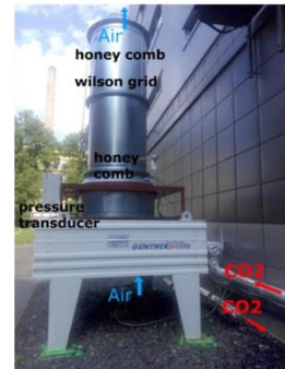
FIG. 8. sCO 2 -HeRo heat rejection unit during test at UJV, Rez.
