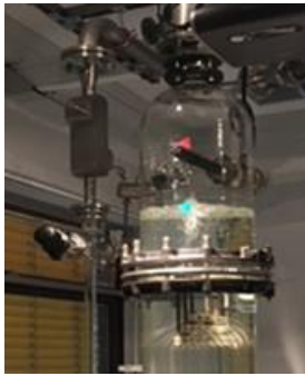
FIG. 6. sCO 2 -compact heat exchanger attached to glass model.
