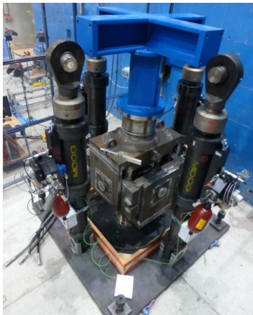
FIG. 5. Full scale pipeline expansion joint during seismic tests at the ELSA laboratory of the JRC of Ispra.
