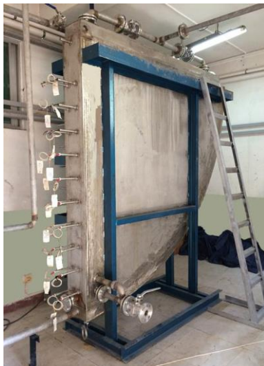
FIG. 2. COPRA test facility in Xi'an Jiaotong University to study melt behaviour in the RPV lower plenum.
