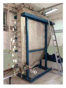
FIG. 2. COPRA test facility in Xi'an Jiatong University to study melt behaviour in the RPV lower plenum.
