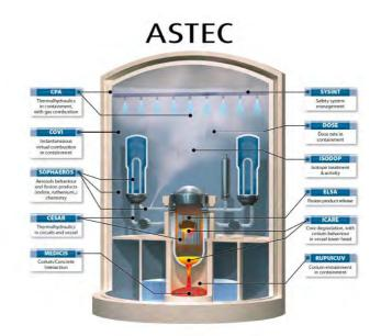
FIG. 3. ASTEC integral code for simulation of severe accidents.
