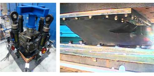
FIG. 5. Full scale pipeline expansion joint during seismic tests at the ELSA laboratory of the JRC of Ispra.
