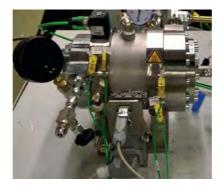
FIG. 6. sCO2-compact heat exchanger attached to glass model.
